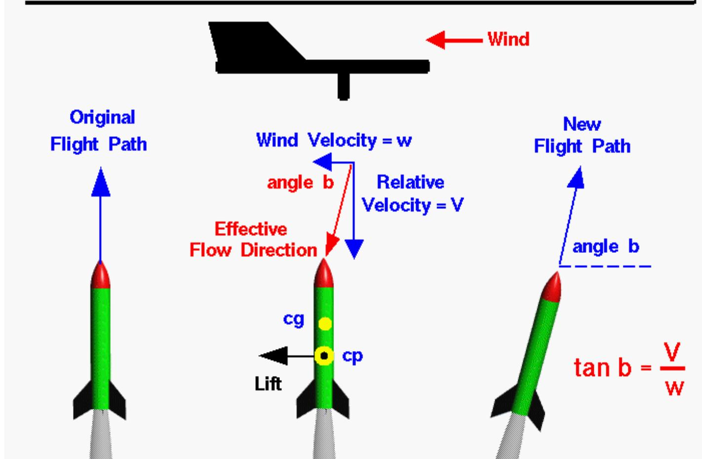
Rockets with higher thrust motors get off the pad faster and have a higher  $V =$  velocity when they clear the launch device, so they are less vulnerable to weathercocking in wind. Using long (6-foot) and rigid launch devices (rails) gives the rocket more time to build up velocity.
