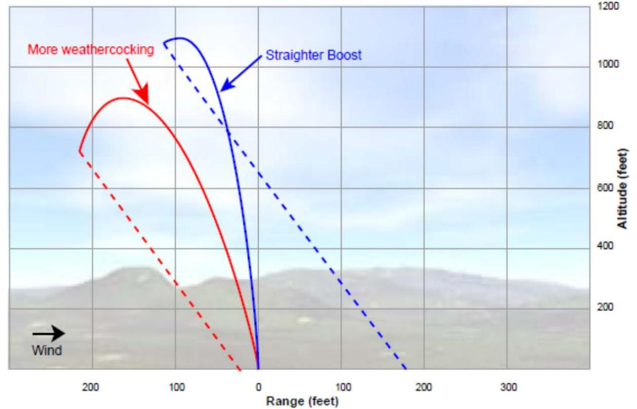
Rockets that weathercock into the wind lose altitude because they do not fly exactly vertically. Angle the launch device in the opposite direction from the wind (away from it) to compensate and get a vertical flight. Figure out the amount of angle needed vs wind speed for your rocket in your test flights by taking data.
